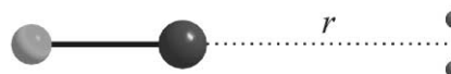
Fig. 2 Definition of the reaction coordinate r used in the calculations as the distance between the M atom (M = Ga or In) in MCl and the centroid of the H 2 molecule.
